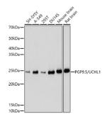
Western blot analysis of various lysates using PGP9.5/UCHL1 Antibody at 1/1000 dilution. Secondary antibody: HRP-conjugated Goat anti-Rabbit IgG (H+L) at 1/10000 dilution. Lysates/proteins: 25  $\mu$ g per lane. Blocking buffer: 3% nonfat dry milk in TBST. Exposure time: 1s.
