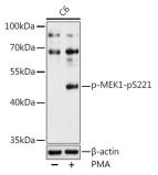
Western blot analysis of lysates from C6 cells, using Phospho-MEK1-pS221 Antibody at 1/1000 dilution. C6 cells were treated by PMA/TPA (200 nM) at 37 °C for 30 minutes after serum-starvation overnight. Secondary antibody: HRP-conjugated Goat anti-Rabbit IgG (H+L) at 1/10000 dilution. Lysates/proteins: 25  $\mu$ g per lane. Blocking buffer: 3% nonfat dry milk in TBST. Exposure time: 60s.
